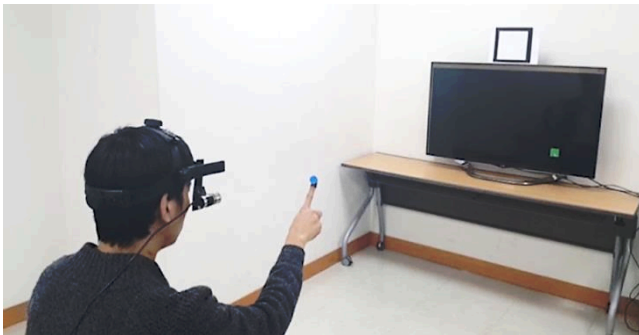
Figure 2: The setup for the experimental target selecting demo: user wears the head mounted camera and the color marker on the fingertip and selects an object at a fixed depth appearing on the monitor.
