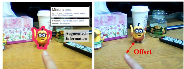
Figure 1: Blurry (Sticky) Finger: proprioceptive pointing and selection, using the finger to point at (and even segment) the target object but without focusing on it (thus blurred) and, relying upon the proprioceptive sense (user view, left). Due to the difference in the positions of the user eye and camera, there is an offset that must be corrected to identify the intended target point in the camera view (right).
