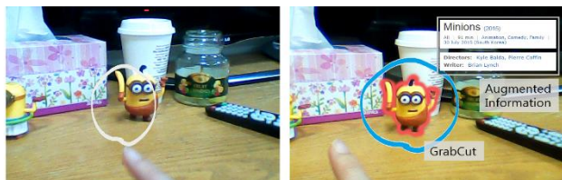
Figure 1: Proprioceptive pointing and selection: using the finger to point at the target object but without focusing on it and, relying upon the proprioceptive sense. The error between the camera and eye view is resolved to correctly segment out the target.
